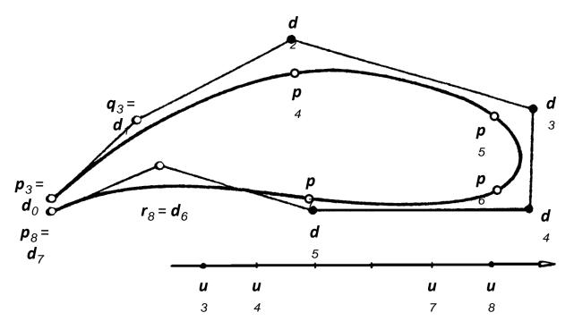
Endpoints  $p_3 = d_0$  and  $p_8 = d_7$  as well as tangents ( $q_a = d_1$  and  $r_b = d_6$ ) have to be preset
